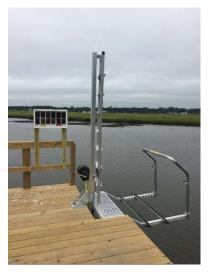
**Before you start -** To use the kayak launch by yourself, you must be able to raise and lower the lift using the winch mechanism. Turing in one direction lowers the lift, turning in the opposite direction raises it. You must also be able to climb up and down the attached ladder.
